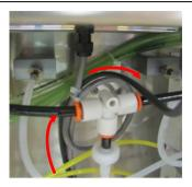
29. Slide the black nut onto the In-Line heater cable and insert the cable through the explosion proof fitting on the underside of the Electrical Enclosure on the right side (Below HR wire connector).
