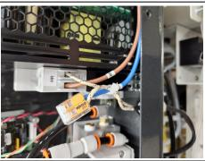
36. Place a cable tie around the black In-Line Heater cable and the gray Pressure Sensor cable. Carefully cut off excess from the cable tie without damaging any insulation.
