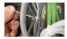
26. On the lower end of the same set of tied cables from the step above, cable tie the 6 cables to the 1 control box cable. There should be 7 cables altogether. Carefully trim excess cable tie without damaging any insulation.
