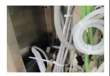
27. Slide two Z462 cable holders onto the In-Line Heater cable (Blue Arrows). Insert the cable holders onto the 2 PEM studs underneath the In-Line Heater (Red Arrows). Screw the two remaining nuts back on, securing the bracket. make sure the star washers are facing inside.
