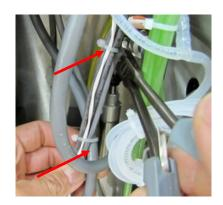
11. Pull the white thermistor cable out of the large grommet in the left gusset panel when facing the back of the instrument.
