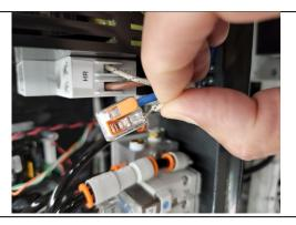
14. Use a small flathead screwdriver to *loosen* the In-Line Heater conductor going to the Heater Relay, labeled "HR" (Screw should not come all the way out).
