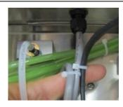
32. Insert one of the wires from the In-Line Heater cable and the loose blue cable into each side of the Splicing Connector. Gently tug on the wires to ensure a secure connection.
