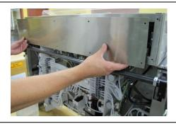
2. Unscrew the 7 screws on the stainless steel top panel and remove. Set screws and panel aside for reattachment later.
