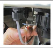
10. Carefully cut off both cable ties connecting the white thermistor cable to the gray cables on the left side of the back of the instrument without damaging the insulation.
