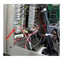
7. Using a dental pick or a small screwdriver, depress the tabs (Black Arrow) inside the J10 connector in order to slide the two conductor out of the terminals (Red Arrows). Set aside the white J10 connector for later use.
