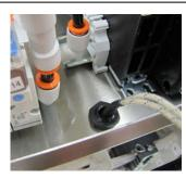
31. Use a cable tie to secure the black In-Line Heater cable to the gray pump motor cable as it was earlier on. Carefully cut off the excess from the cable tie.
