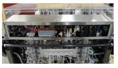
3. Unscrew the 6 acorn nuts securing the clear back plastic panel and remove. Set aside for reattachment later.
