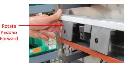
c. Looking straight down on paddle #5, measure the distance that the bottom edge of this paddle extends beyond the orange gasket. This distance should be 4/32" - 5/32". If this distance is not correct contact ANKOM Technology for instructions on how to make an adjustment. Note: The gasket can be either Orange or Black.
