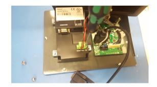
4. Pull the light green connector from the socket.
