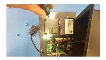
6. Push the broken touch screen display out from the rear. Slide the new one back in place and be sure the front flange sits flat against the front of the controller front panel.
