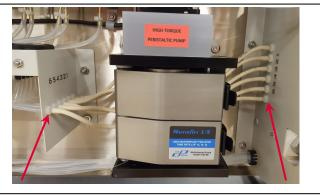
2. Open the Pump doors by pulling on the two latches on the right side of the pump, allowing access to the pump tubing.
