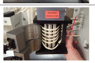
4. Obtain the TDF99 Long-life Pump Tube Replacement Set. Note that one spare set comes with a new TDF analyzer. Additional TDF99 Pump Tube Replacement Sets can be purchased on line at www.ankom.com or call: 1-315-986-8090.
