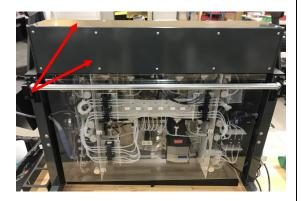
2. The 12-Station Manifold (Red Bracket) is located in front of the "I/O1" circuit board. The 12 solenoid valves are each labeled and solenoid #1 is identified by the green arrow.
