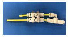
6. On the underside of the electrical enclosure, disconnect the 8215 Yellow Polyurethane Tubing in the leftmost position (as viewed from back of instrument). This tube is about 21" in length and goes to the mixer piston. Remove it and insert the 2½" piece of 8215 Tubing from the TDF113 Mixer Flow Control Valve Assembly (Red Arrow). Gently tug at the tubing to make sure there is a good connection.
