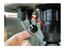
7. Pull the white thermistor cable completely out of the black fitting and set aside nut for later use.
