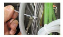
21. On the lower end of the same set of tied cables from the step above, cable tie the 6 cables to the 1 control box cable. There should be 7 cables altogether. Carefully trim excess cable tie without damaging any insulation.
