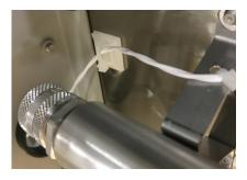
16. Feed the white thermistor cable through the large grommet on the left side gusset panel (When facing back of instrument).
