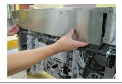
2. Unscrew the 7 screws on the top panel and remove. Set screws and panel aside for reattachment later.
