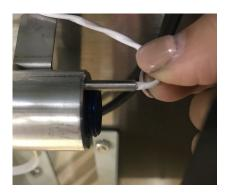
14. Use cable ties to reattach the thermistor wire to the two upper brackets of the In-Line Heater.
