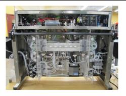
4. Detach the white 3-pin connector labeled "J10" from the MUX-T circuit board.
