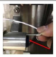
12. Obtain the new TDF98 Thermistor Assembly. The white 3-pin connector should come labeled "J10".
