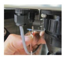
8. Carefully cut off both cable ties connecting the white thermistor cable to the gray cables on the left side of the back of the instrument without damaging the insulation.
