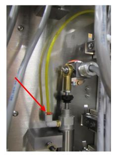
3. Unscrew the 8265 Shoulder Screw from the top of the Mixer Piston using an 1/8" hex wrench.
