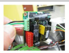
14. Install the new 8301 Stepper Motor Controller on the inside of the Electrical Enclosure. Tighten the four 8035 Male-Female Stand-offs firmly by hand and only an additional ¼ turn with a ¼" socket wrench. Loosely finger-tighten each one until all four are aligned then snug them lightly once they are in place. Do not over-tighten as the threaded ends can break off. Connect the two 8-pin connectors onto the Motor Controller board (see arrows).
