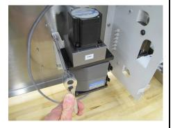
Install the new High Torque Pump Motor assembly in the same location. Replacement screws, nuts and gaskets are provided in case any have been damaged.
