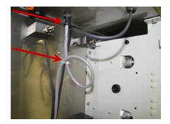
3. Remove top and back panel to the electrical enclosure. A 1/8" Allen wrench driver is needed. One was provided with the instrument on the original purchase.
