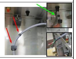
12. Take the new Fan and Bracket assembly and install it as shown using the 1 inch hex stand-offs removed earlier. Tighten these with a 1/4" hex driver. Note that the picture is as viewed from the rear of the instrument.
