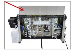
4. Identify the Motor Controller within the electrical enclosure. Use an antistatic wrist strap grounded to one of the studs within the electrical enclosure to eliminate static discharge when working around the circuit boards.
