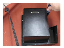
22. Install the new TDF99 Pump tubes into the peristaltic pump following service Procedure TS028 which accompanies the tube sets. Follow the step in TS028 which describe the break-in process and running of volume calibration. With all this completed, the instrument is ready to be returned to service.
