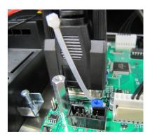
21. Close the control panel back up and secure with the six acorn nuts removed earlier. Reattach this to the instrument and plug in the connector to the back. Also close up the back of the electrical enclosure removed in step 3.
