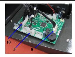
18. Finger-tighten the four standoffs onto the four PEM studs to secure the board. Use a ¼" socket. As needed, tighten or loosen the two stand-offs near the micro-switches on the circuit board to obtain the appropriate sensitivity of the push-button micro-switch through the front decal.
