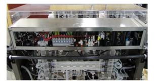
3. Identify the Paddle Heater Relay (part 8338—Red Arrow) within the electrical enclosure. Note: Some instruments have two in-line fuses as shown (Yellow Arrow).
