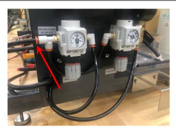
2. Disconnect the other two nitrogen lines at the regulator as marked with the red arrows.
