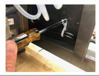
5. Free the cable strap from the back side of the screw.
