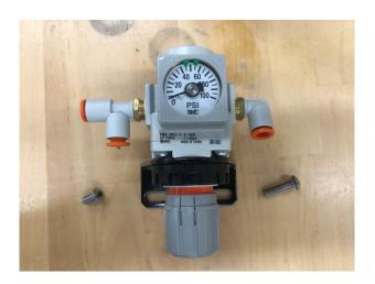
8. Install the new TDF61 High Pressure Regulator with the short (%") screw on the left and the longer (34") screw on the right.
