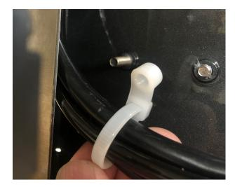
6. Using an 1/8" Hex Driver, remove the two screws holding the TDF62 Low Pressure Regulator in place.
