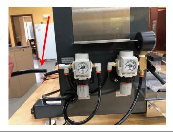
2. Disconnect the other two nitrogen lines on the low pressure regulator as marked with the red arrows.
