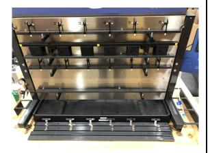
2. Remove the two Service Access screws on the left and right sides of the front of the instrument.
