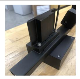
17. Feed the paddle cable connector through the large hole in the front of the instrument.
