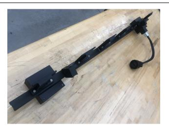
9. Remove the two screws holding the paddle to the paddle bar, using a 7/64" hex wrench.
