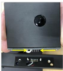
14. Use the two alignment screws as a guide aligning them with the receiving holes in the paddle, keeping the paddle vertically straight. Gently connect the pins and evenly press the paddle down and in position until the paddle meets the gasket.
