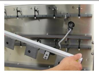
8. Set the paddle bar upside down on approximately 1/2" blocks to keep it stationary. This is important to maintain proper positioning of the 5-pin connector within paddle to the receiving part within the paddle bar.
