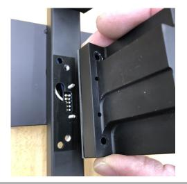
12. Position a new paddle gasket in place over the interface of the paddle and paddle bar. Be sure to align the holes in the new gasket with those of the paddle bar. Gasket might look slightly different.
