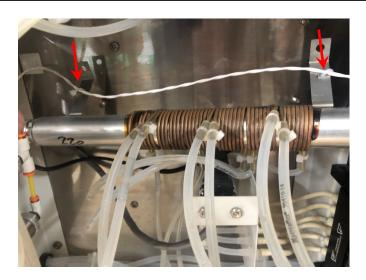
24. Connect the twelve new tubes from the in-line heater to the barbed fittings on the tubing support panel and onto the pressure sensor assembly. Note: Orient the lower tube so that the tube on the left of the in-line heater is connected to the pressure sensor t-connector furthest from the front of the instrument. Then as you work your way through the other tubes to the right on the in-line heater choose the t-connector next closer to the front of the instrument.
