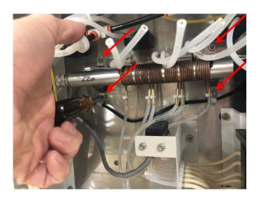
6. Pull the in-line heater assembly off of the four threaded studs on the front panel.
