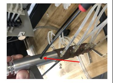
9. Unscrew the knurled nut holding the heater cable and pull the rubber stopper from its position so that the heater cartridge inside is now loose.
