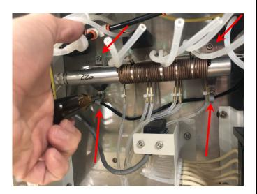
22. Resecure the in-line heater power cord to the pressure sensor assembly cable with a cable tie.
