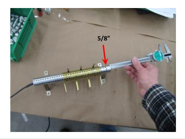
17. With the heater cartridge held in this position, secure it in place with a 3/32" hex wrench.
