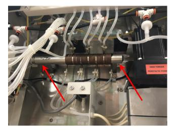
2. Disconnect the twelve tubes going to the tubing support panel (above) and to the pressure sensor assembly (below).
