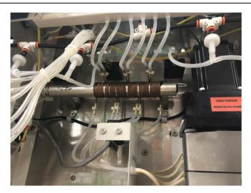
25. Plug the ANKOM<sup>TDF</sup> instrument back in and turn the power on. Go to Diagnostics and select Pump Tube Test. Use the TDF70 Flush Tube assembly to connect all of the fluid ports to a filled Deionized Water container.
