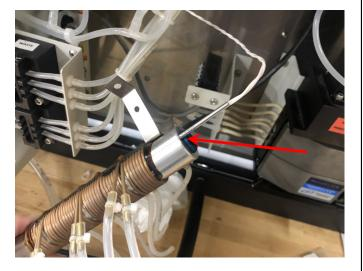
8. Loosen the set screw on the in-line heater with a 3/32" hex wrench. This set screw holds the heater cartridge in place and MUST be loosened before proceeding to the next step to avoid damage to the power cord.
