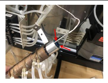
21. Return the in-line heater brackets to the four threaded studs on the front panel in the orientation shown. On the lower two nuts reinstall the cable restraints and attach these to the threaded stud before replacing the nuts. Tighten the four nuts with a 3/8" nut driver or socket wrench.
