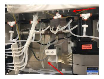
3. Carefully cut the cable ties holding the white thermistor wire to the two brackets on the in-line heater.
