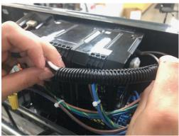
11. Place a zip tie through the white zip tie fastener on the side of power supply A and loosely tighten around the wires being held by the black wire sleeve. Cut off zip tie excess.
