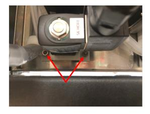
15. Place the black cable holder which is holding the temperature sensor tube onto the stud on the top right of the bracket (blue arrow). Then place the 167 Hex Nuts onto the top right and top left studs and tighten with a %" socket wrench (red arrow).
