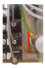
17. Reconnect the delivery tubes coming from the reservoirs: Water (W), Buffer (B), EtOH78 (78) and EtOH95 (95) to the left side of the supply valves.
