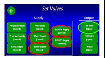
21. Press GO and confirm that approximately 10 mls of the specified solution has been delivered through the IDF fill nozzles and into the beakers. Confirm that the valve(s) being tested are opening also by observing that the vacuum reading (max) is in the -0.8 to -3.0 psi
