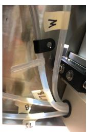
Using a ¾" socket wrench, remove the two 167 Hex Nuts from the top left and the top right corner of the TDF25 Supply Valve Bracket.
