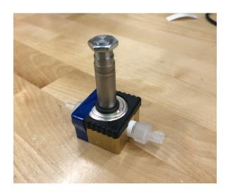
12. Use a screwdriver to fasten the new TDF25.5 Supply Valve Body & Piston back onto the TDF25 Supply Valve Bracket with the 114 Panhead Bolts. Orient the new valve bodies in the same way as the ones removed.
