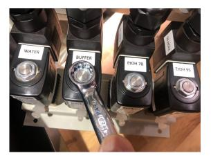
14. Place the TDF25 Supply Valve Assembly back onto the studs on the front panel of the TDF Instrument. Use a ¾" socket wrench to tighten two 167 Hex Nuts on the bottom left and the bottom right corners.
