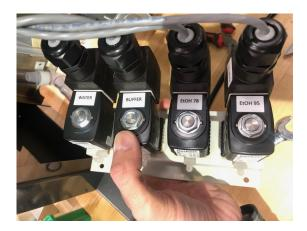
9. Use a 9/16" wrench to loosen and remove the nut on top of the valve you are replacing. Once the nut is removed you can pull off the valve body from the brass bottom.
