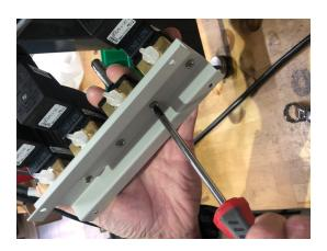
11. Obtain the new TDF25.5 Supply Valve Body & Piston Assembly. remove the blue tape and the nut on the top.
