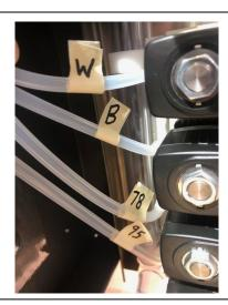
5. Repeat step 3 & 4 with the four silicone tubes on the right side of the TDF25 Supply Valve Assembly. The four tubes should be labeled as follows:
