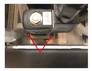
8. Once all four hex nuts are off, you can remove the TDF25 Supply Valve Assembly from the front panel of the TDF Instrument.
