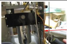
13 Replace the two screws to secure the Fill Cup Assembly bracket to the frame.
