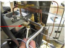
8. Unscrew the Q7 Valve base and fittings. Use a wrench on the T-fitting as shown.
