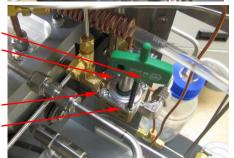
2. Loosen the two compression nuts on the 1/4" stainless tube coming off of the Q7 valve base.
