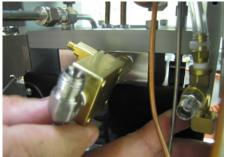
11 Replace the small 1/4" tube going from the Q7 Valve to the Vent Valve. Finger tighten only, initially.
