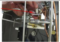
b. Replace the four screws securing the valve stem with a T20 Torx screwdriver.
