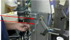
2. Loosen the compression nut to remove the Vent Trap Assembly. Remove and set aside for later.
