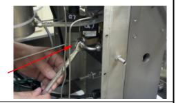
8. Reconnect the Vent Trap Assembly by tightening the compression fitting.
