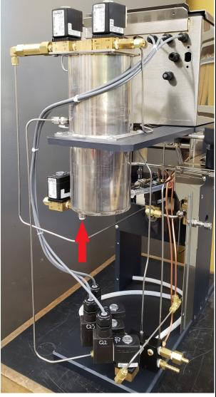
**3.** Use a 3/16" Allen wrench to remove the Drain plug. Be sure to have a beaker readily available to Catch the solvent with a beaker.
