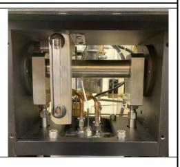
4. Viewing from the back panel, cut the zip ties from the Sight Glass Assembly's tri-fold tubing.
