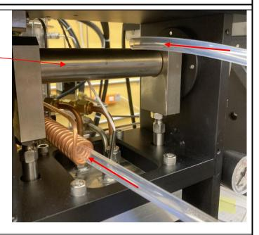
10. Install the new tubes over their correlating connections. Then, install new zip ties.
