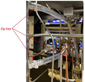
5. Use a boxcutter to cut small slits in the tubing to remove all three from their connections.
