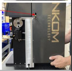
Remove the front plate by unscrewing the four attachment screws with a 1/8inch Allen wrench. Set the screws aside.
