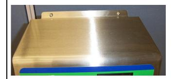
5. Remove the two Allen screws securing the electrical cover closed. Open to access the electrical compartment.
