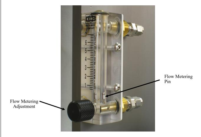
5. Turn the (Flow Metering Adjustment) black knob to regulate the flow to between 6 and 7 on the flow scale. You will adjust the flow when the water is continuously on. If you have any questions please contact ANKOM at (315) 986-8090.
