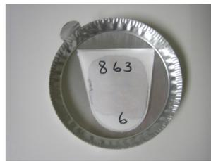
**After removing the Filter Bag from the oven, is each bag weighed with its tin or weighed separately?** The Filter Bags and tins are weighed together. If the Filter Bag is removed from the weigh tin, prior to weighing, some residual fat may remain in the weigh tin and will not be accounted for.
