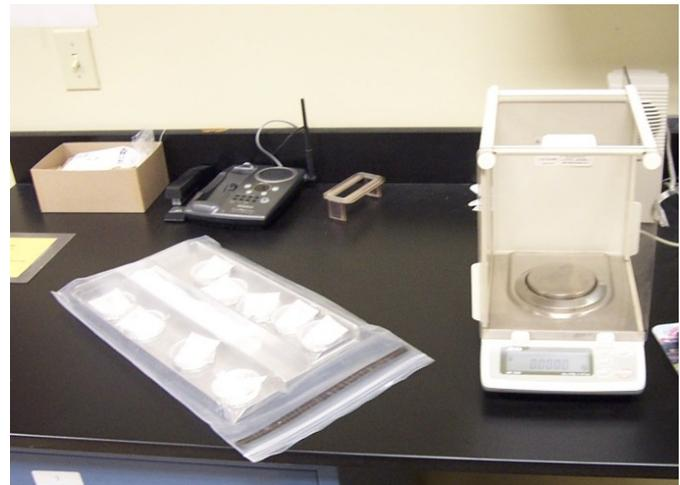
2. Allow 10-15 minutes to cool to room temperature. Open the magnetic strip and slide one tray out of the pouch far enough to remove one tin. Weigh the tin and bag. Leave the bag open.
