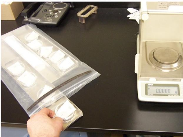
3. Slide the tray out to get the next sample and continue weighing in this manner. Ambient air will not affect the other samples because the air is not being pushed into the pouch as it is when opening and closing a desiccator.
