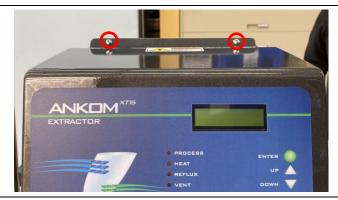
Remove the control panel plate cover by removing the screws with a small Phillips screwdriver. Set aside the plate cover and screws to be reassembled later.
